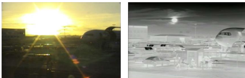
Images facing sun from visible light camera (left) and from thermal camera (right)
